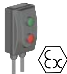
This device using SSRs controls AC motors in hazardous area. Control by push-buttons with embedded magnet actuating Reed switches.
